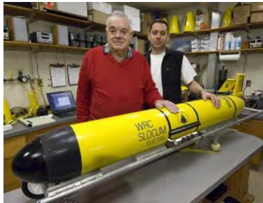
autonomous vehicle, propelled by buoyancy changes rather than a propeller. In 1994 he was granted a patent for a unique thermal engine which used energy harvested from oceanic temperature differences to propel the glider.
