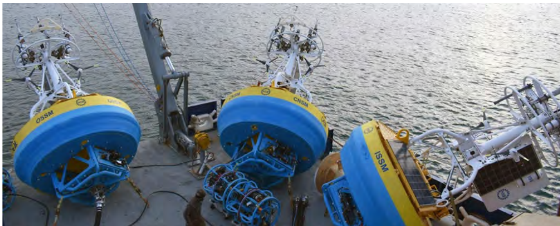
Ocean Observatories Initiative (OOI) surface buoys awaiting deployment in the Irminger Sea. Credit: Rebecca Travis © Woods Hole Oceanographic Institution.
