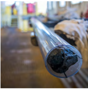
A drill core is brought on board the Joides Resolution for scientific analysis. Photo: Sandra Herrmann (IODP/JRSO)
