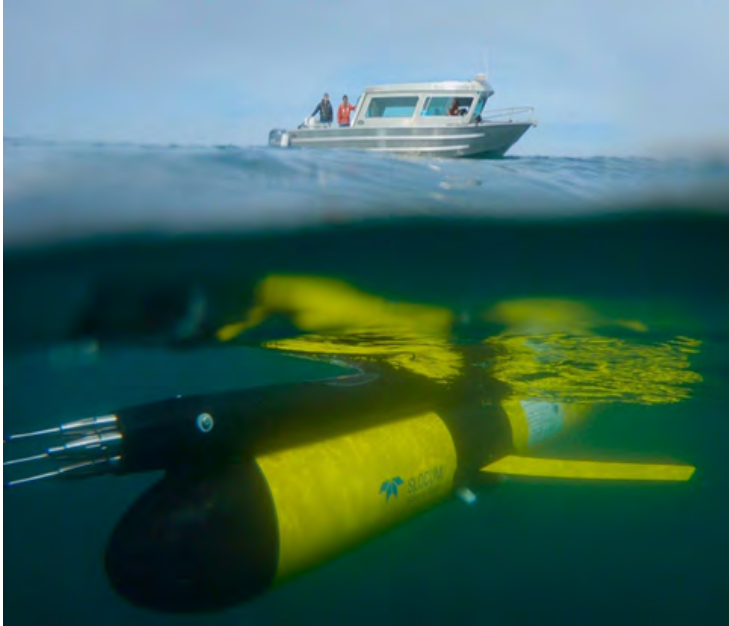
Figure 4: Ocean glider Mike (short for Mike Rorider, in reference to the Rockland MicroRider turbulence sensor the instrument carries) during deployment by the Hakai Institute Oceanography team in June 2019. Photo credit: Hakai Media, Katrina Pyne.
