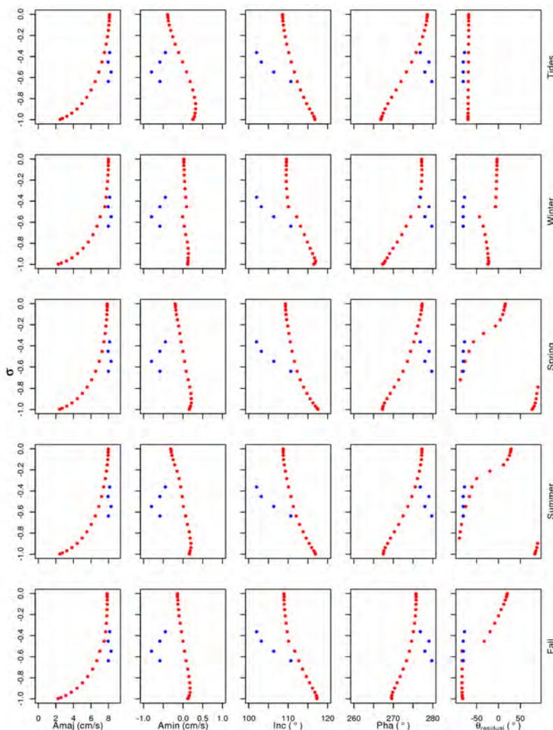
Figure 3. Comparison between the M2 constituent results from the tidal analysis of currents from ADCP deployment 531 (blue) and the FVCOM model (red). Shown are the amplitudes of the M2 tide along the major and minor axis of the current, the inclination (Inc) of the major axis, the phase (Pha) and the direction from the principal component analysis of the residual currents ( $\theta_{\text{residual}}$ ). The vertical coordinate,  $\sigma$ , varies from 0 at the surface to -1 at the seabed.
