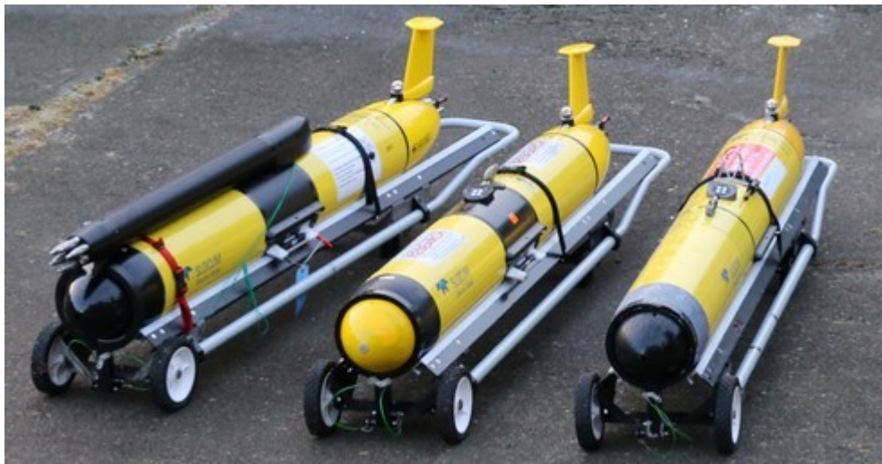
Figure 3: 'The fleet', from left to right: Slocum glider with Microrider, oxygen, fluorescence, and backscatter sensors, and CTD. Capacity to dive to 1000m; Slocum glider with irradiance, oxygen, and backscatter sensors, and CTD. Capacity to dive to 350m; Slocum glider with echosounder, CTD, and acoustic capabilities (DMON not shown, see Figure 1). Capacity to 200m. Note wings, to balance pitch and roll, are missing. (Photo credit Whale Lab, UVIC).
