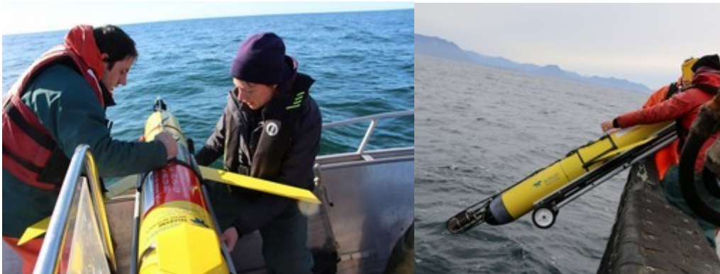
Figure 1: Glider deployment from March 2016 (L) and February 2017 (R). The DMON is visible protruding ahead of the nose of the glider (Photo credit: Whale Lab, Uvic).
