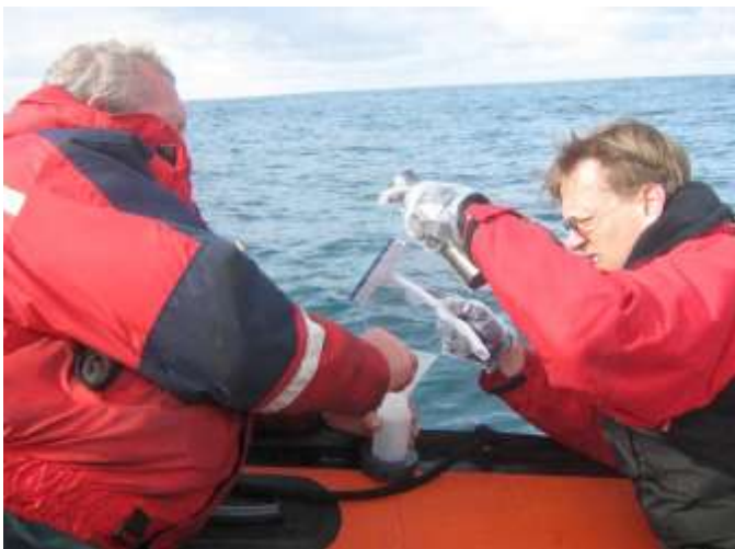
SML sampling with the glass Plate technique. Photo: SCOR
