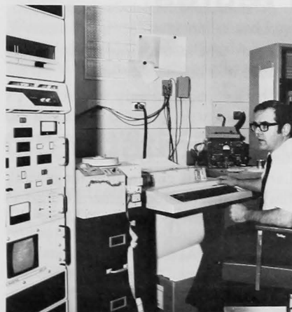
Author Ken Devine surveys the ADRES system, including minicomputer, paper tape reader punch, printing terminal and equipment rack, all standard gear in upper air stations. (Applied Photo)
