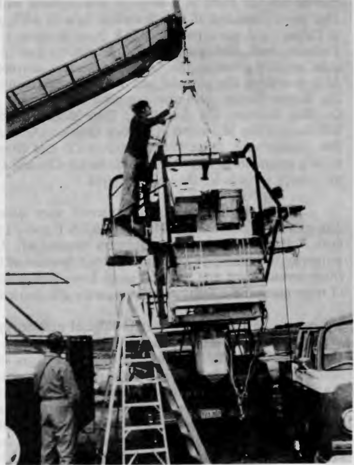
Stratoprobe III Payload, fourteen instrument systems plus two on-board cameras.
