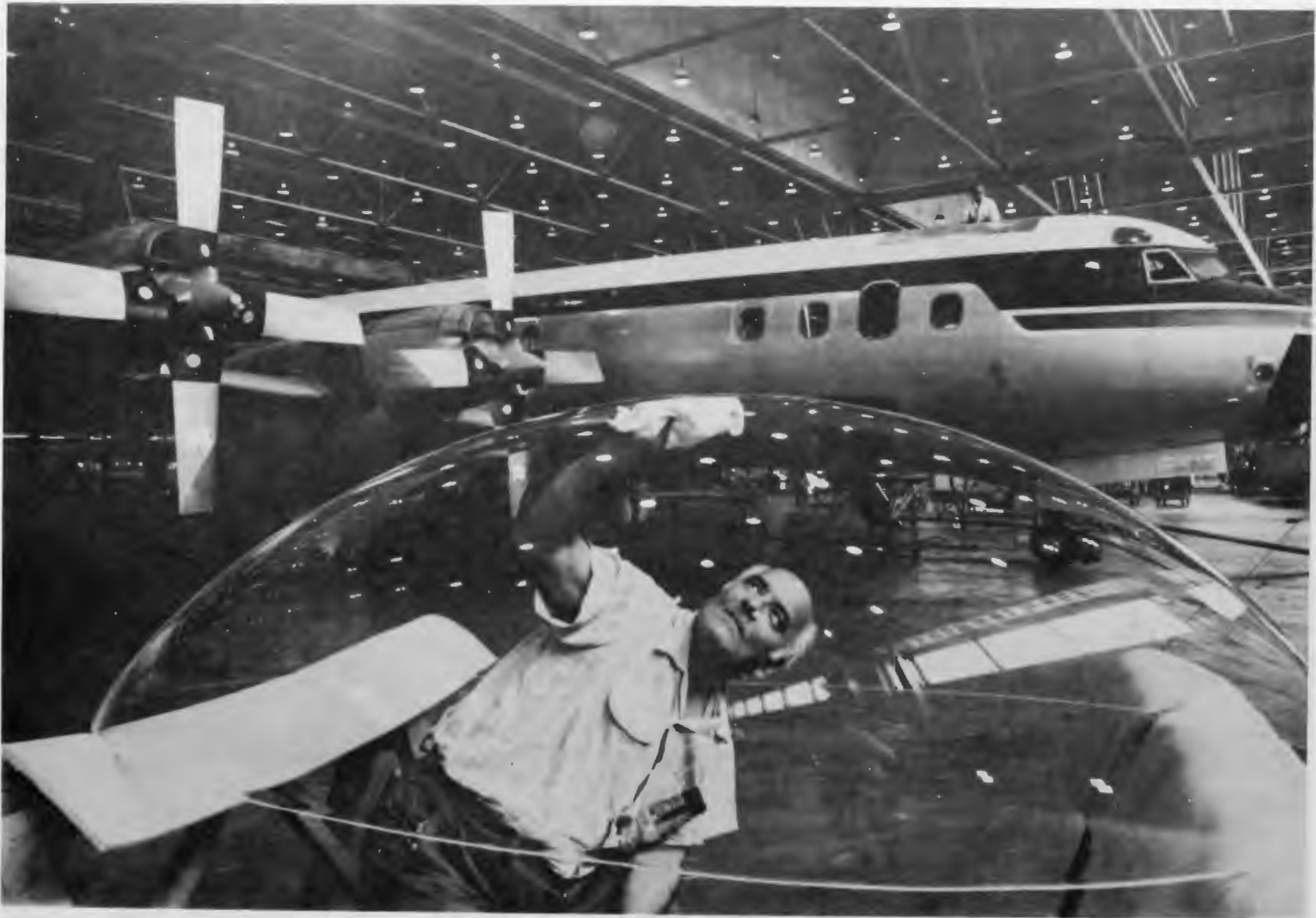
Figure II: The plexiglass dome is being prepared for installation on the upper side of the aircraft fuselage. A workman can be observed positioned in the opening over which the dome will be placed (background).
