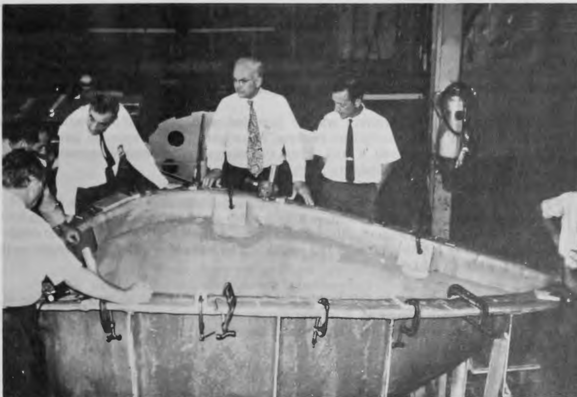
Figure III: The mould prepared for formation of the 12' radome for the radar antenna is examined during an inspection tour.
