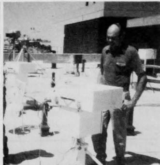
Also displayed is the AES designed Brewer spectrometer, one of the world's major ozone detecting devices. Technologist Archie Asbridge stands by.
