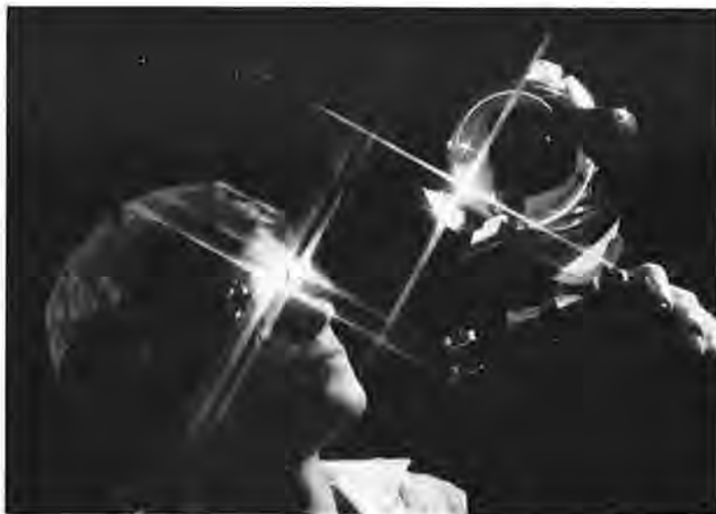
The author checks the Campbell-Stokes sunshine recorder. The glass sphere focuses the sun's rays on a strip of treated paper, burning a path to record the hours of bright sunshine.
