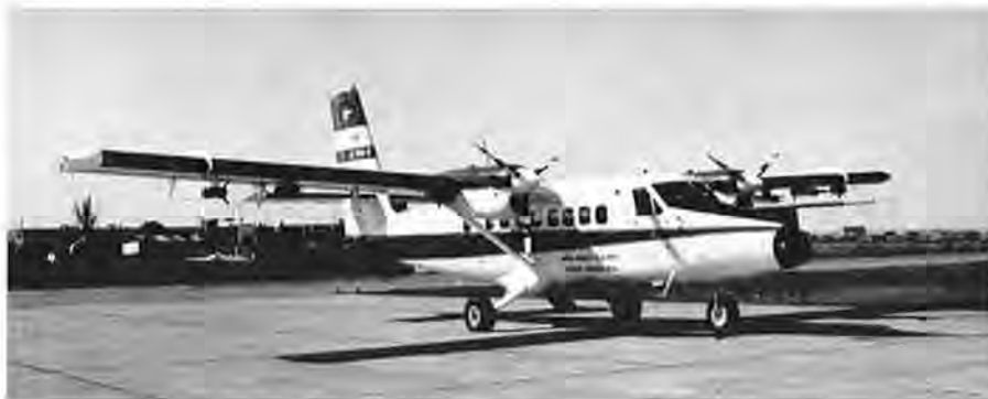
Figure 4 Twin Otter instrumented aircraft operated by the National Aeronautical Establishment of the National Research Council of Canada (Photograph: Courtesy of the NRC Flight Research Establishment).
