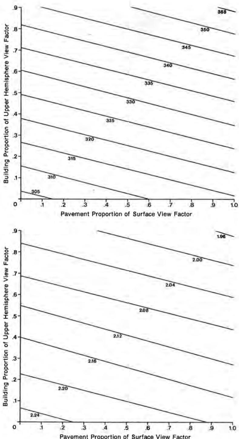
Fig. 1.. Environmental long wave radiation ( $\text{W m}^{-2}$ ) (top) and equilibrium clothing requirement (clo) (bottom) with constant sky radiation.
