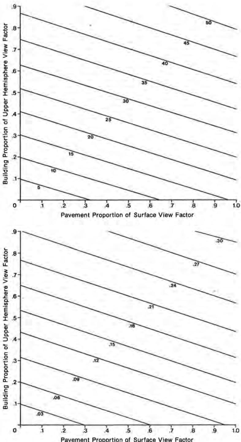
Fig. 2. Difference in environmental long wave radiation ( $\text{W m}^{-2}$ ) (top) and equilibrium clothing requirement (clo) (bottom) from those in an open rural environment, with variable sky radiation.
