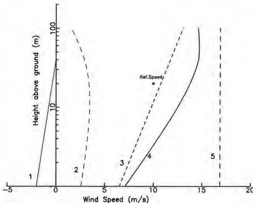
FIGURE 2. Wind speed profiles for sample run with calculations at additional prediction heights.
