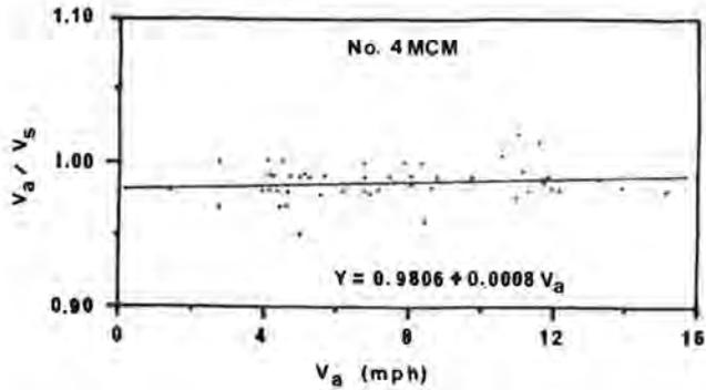
Fig. 1. Sample graphical presentation of anemometer calibration for No. 4MCM.
