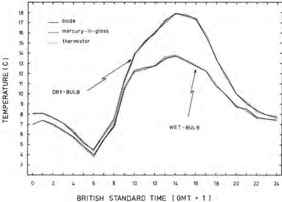
Fig. 6. Daily record of screen wet- and dry-bulb temperatures measured by diode, mercury-in-glass and thermistor thermometers.
