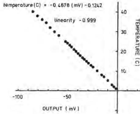
Fig. 5. Typical calibration of thermometer unit as used in the screen.
