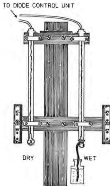
Fig. 2. Diode psychrometer mounted on Stevenson screen thermometer mount.
