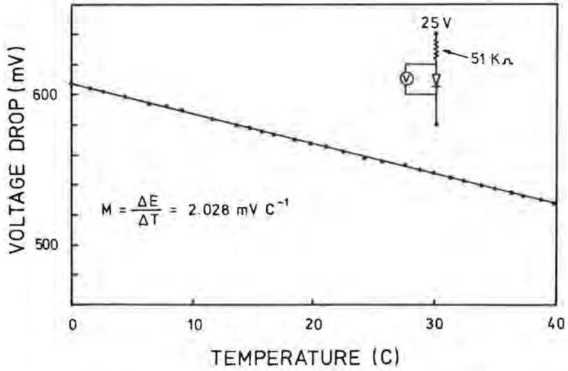
Fig. 1. Typical calibration characteristic of a 1N 4148 diffused silicon diode.
