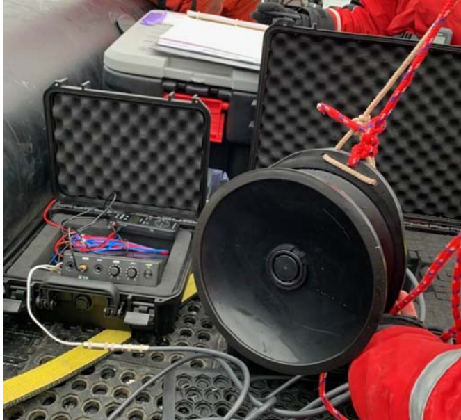
Figure 4. Underwater speaker used to conduct experiments.
