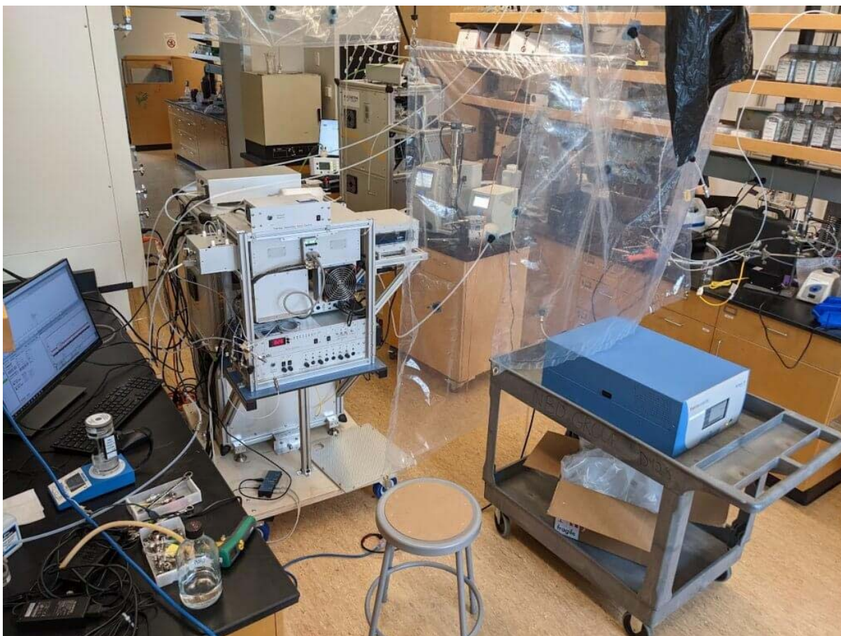
Figure 2. Experimental setup used to study the atmospheric oxidation of volatile organic Se. The Vocus proton-transfer-reaction time-of-flight mass spectrometer can be seen in the center left of this picture.
