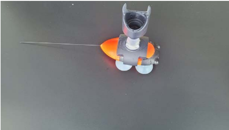
Figure 2. Suction cup hydrophone data logger (DTAG).
