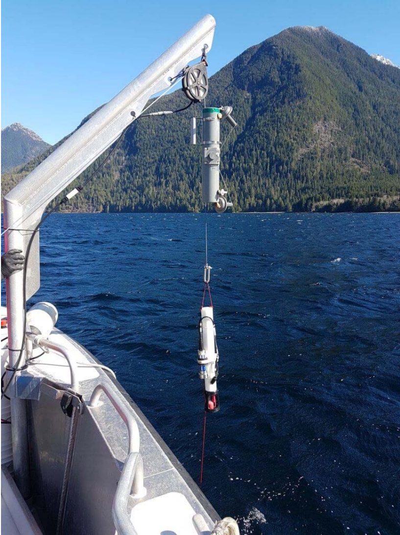
Figure 3: CTD and Niskin deployment off the CME Anderson in Quatsino Sound (photo credit: Glenn Cooper).
