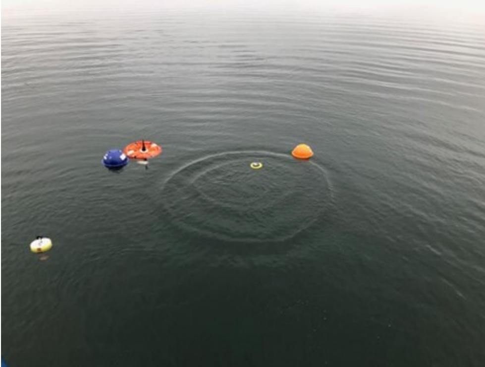
Figure 1: Photo of several drifters just after they were dropped into the St. Lawrence Estuary during the 2020 release experiment. Photo provided by Cédric Chavanne, Oceanographer at UQAR.
