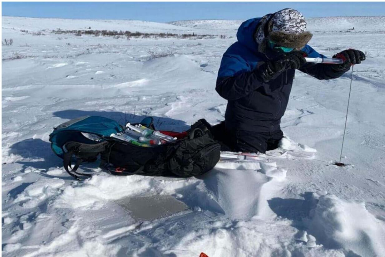
**Image 5: Measurements of Carbon Emissions.** As well as measuring the snowpack properties, we capture CO<sub>2</sub> fluxes that come out of the ground, through the snowpack, and into the air. We do this by placing low-cost gas sensors in the snowpack at different levels or extracting gas samples from the snowpack using a syringe.
