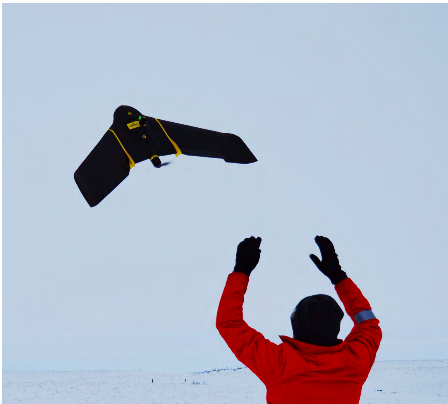
Branden Walker Launching the EBEE RPAS to map snow depth at the Trail Valley Creek Research Basin, NWT. Story Inside p. 16. Photo Credit to Arvids Silis.
