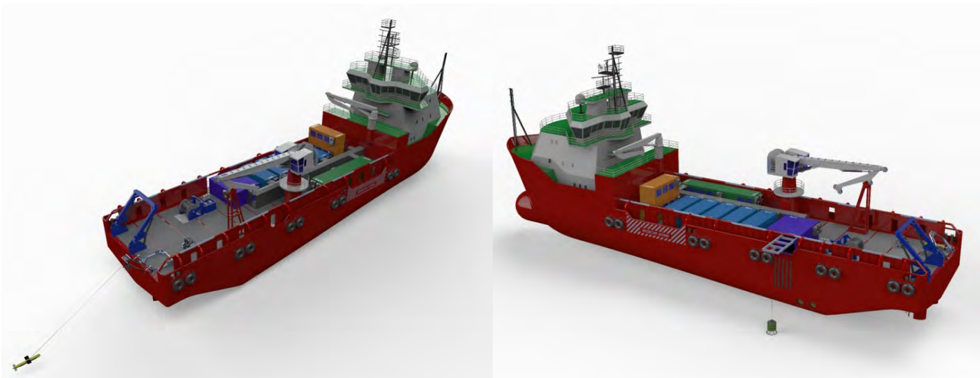
Figure 4. Sketches of a 95m platform supply vessel (PSV) configured with Modular Ocean Research Infrastructure (MORI) including 5 custom laboratories, launch and recovery systems (for CTDs and towed vehicles), extra accommodation “pods”, meeting space and a data processing room. The vessel, as shown, would fall within the “Global” vessel category of Figure 1.
