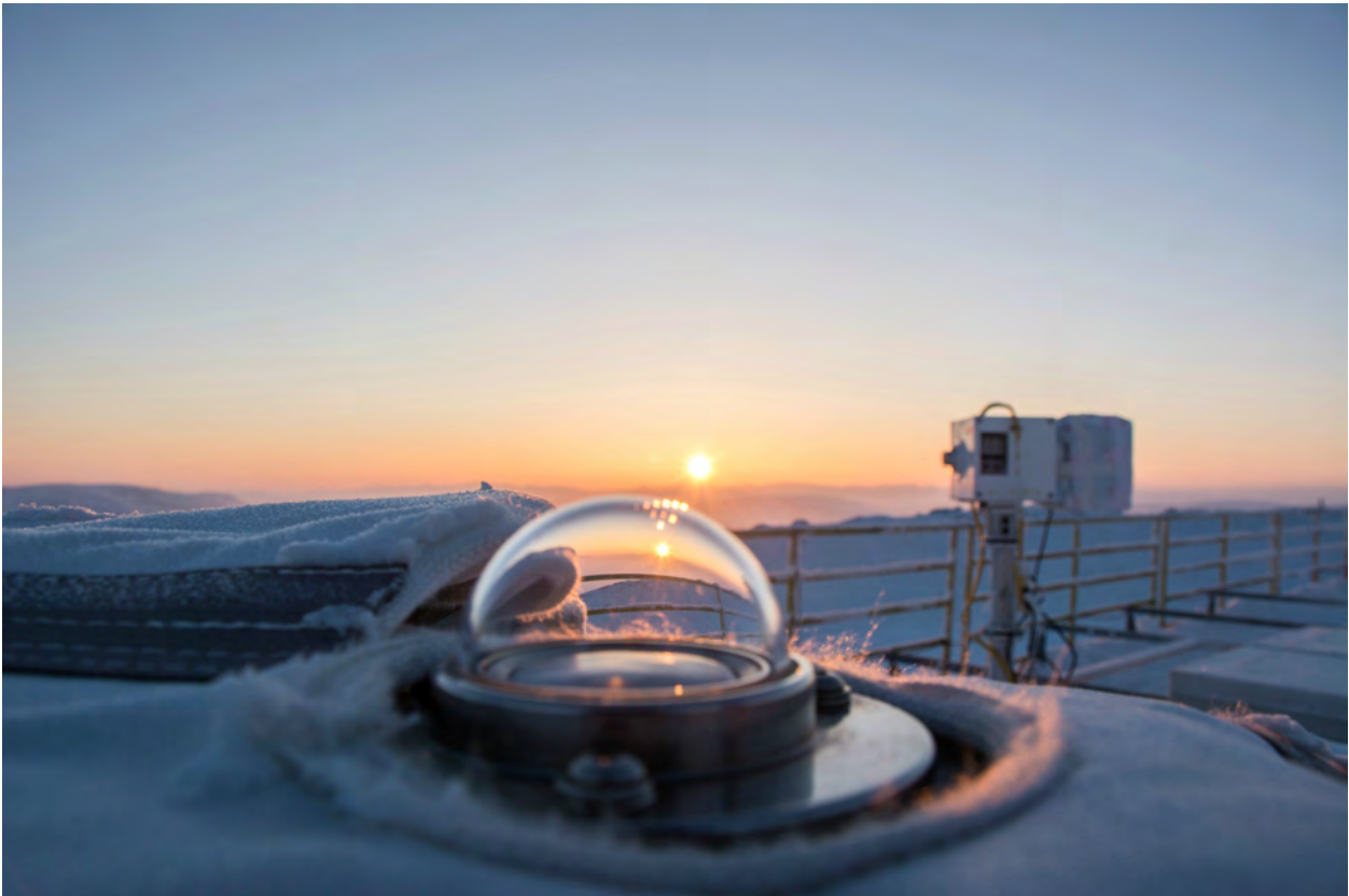
The dome of the PEARL Ridge Lab Brewer spectrophotometer, which measures ozone, in the foreground and the Sun Photo Spectrometer (SPS) instrument in the background on the Ridge Lab roof.
