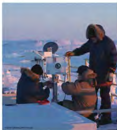
LEFT: Adjusting a Brewer ozone spectrophotometer on the roof of the PEARL Ridge laboratory. PEARL is situated beneath the Polar vortex in winter and that makes it ideal for studying Arctic ozone changes at Polar sunrise, such as the large depletion event seen in Spring of 2011. Photo Credit: Pierre Fogal
