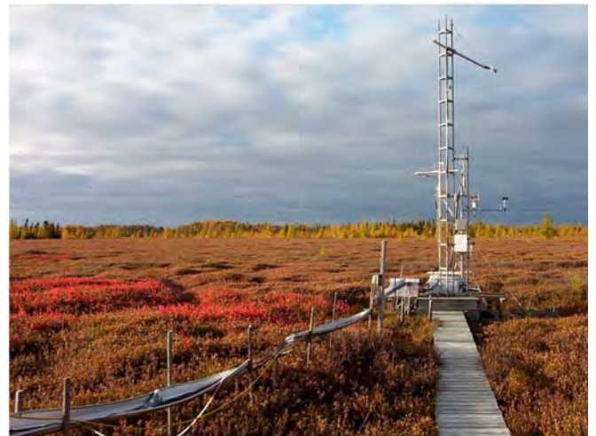
The eddy covariance tower at the Mer Bleue peatland, Eastern Ontario – the longest running carbon observatory for a peatland in the world.
