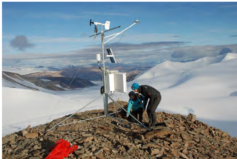
Figure 1: Downloading an automated weather station near the summit of White Glacier, Axel Heiberg Island, Nunavut.
