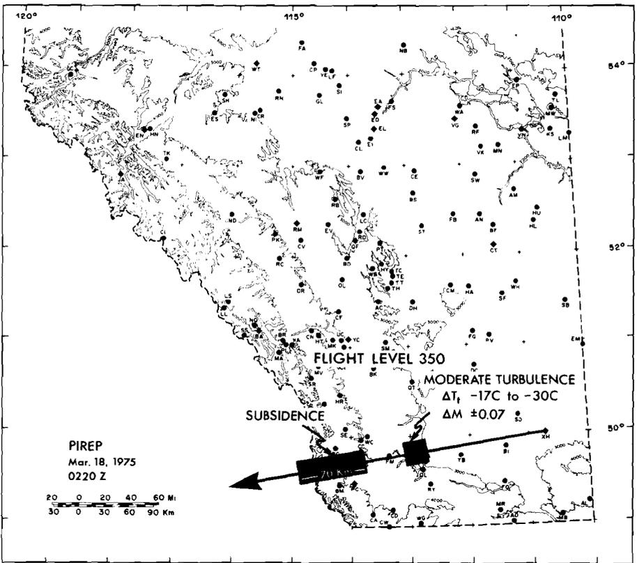
Fig. 2 Commercial jet aircraft pilot report (PIREP) for 0220 GMT, 18 March 1975.  $\Delta T_t$  and  $\Delta M$  indicate, respectively, maximum excursions in total temperature and Mach number during turbulence. "Subsidence" is pilot jargon for a smooth downdraft.
