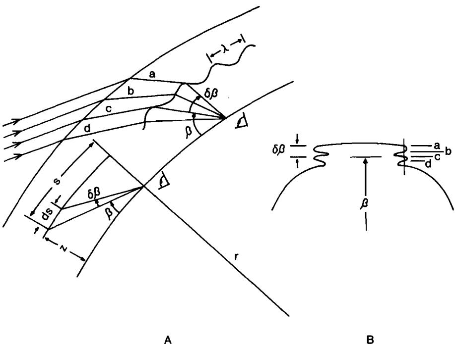
Fig. 4 A. Assume that an inversion at height  $z$  separates two layers of the atmosphere that have different refractive indices. If there is a gravity wave on this inversion surface with wavelength  $\lambda$ , then initially parallel rays of light a, b, c, d (coming from a single point on the sun) can all arrive at the eye. The view as seen by the eye is shown in B. The geometry of the situation is simplified on the left of A for calculative purposes (see Appendix II).
