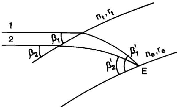
Fig. 7 These are the assumed ray paths through the atmosphere if the theorem is false. The index of refraction  $n$ , and the distances to the center of symmetry (the center of the earth)  $r$  are subscripted  $t$  (for the top of the atmosphere) and  $e$  (for the earth or eye).
