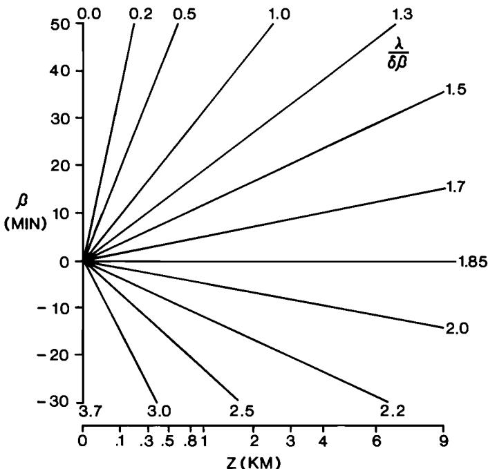
Fig. 5 The function  $\lambda/\delta\beta$  is the ratio of the space wavelength  $\lambda$  in kilometers to the angular wavelength between similar images  $\delta\beta$  in minutes of arc. The height of the inversion above the eye is  $z$  in kilometers and the angular elevation of the images above the astronomical horizon is  $\beta$  in minutes of arc.
