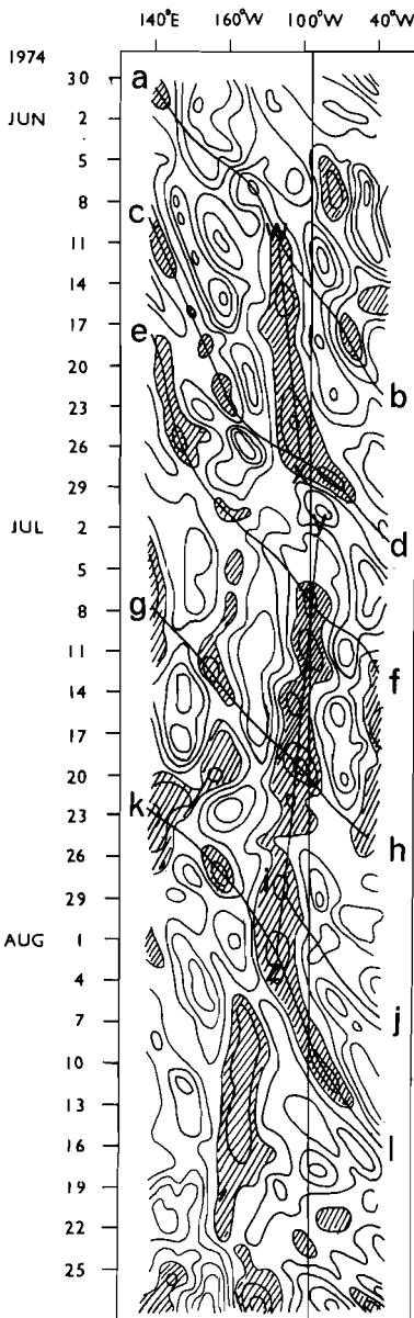
Fig. 3 Hovmöller diagram for 30th May to August 28th 1974. The unlabelled vertical line is the longitude ( $93^{\circ}\text{W}$ ) of the Northwestern Region. Shaded areas are ridges at 500 mb. Unshaded areas are troughs.
