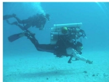
Passing water through a spectrophotometer and a CTD Image credit Ron Zaneveld
