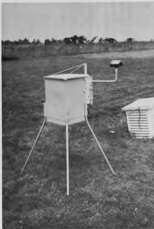
The precipitation sampler installed at Mount Forest, showing the lid in the closed position and, extending out to the right, the sensing head.
