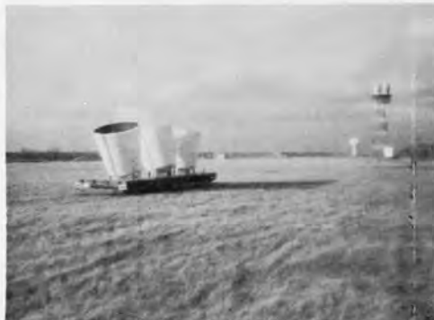
These large horns create an acoustic sounder system with the sound projected upwards and reflected back from clouds. The result is recorded and processed by a computer. The horns have been used on and off for environmental and pollution studies.
