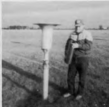
Mr. Chirka also runs a Climate Station on the farm. He is seen here with a Nipher snow gauge that collects snow, which is then melted and measured in a graduate tube.
