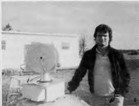
Still very active, however, is this solar radiation suntracker operated here by technician David Barton of Experimental Studies Division.
