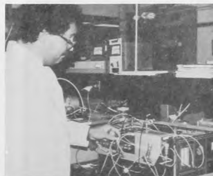
This analyser measures nitrous oxide in the atmosphere. It is an industrial model altered by AES for its own use to improve sensitivity. The alterations are experimental and the analyser is often used in chemical process research studies. Spaghetti anyone?
