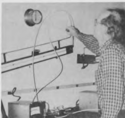
Chemist Dr. Al Wiebe adjusts this inclined manometer, an instrument used to calibrate mass flow meters which record air volumes and air flow rates.
