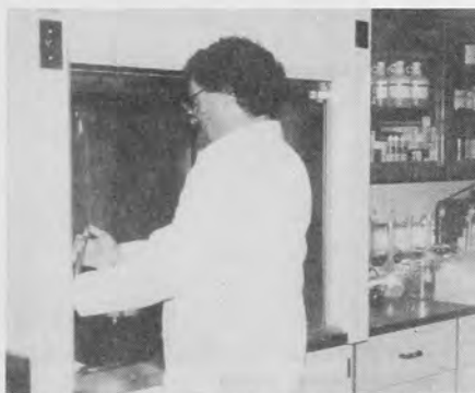
Another more frequently used safety device is the stainless steel fume-hood. The furnace-like shield supplies an airflow to the outside which prevents scientists from breathing in chemical fumes.
