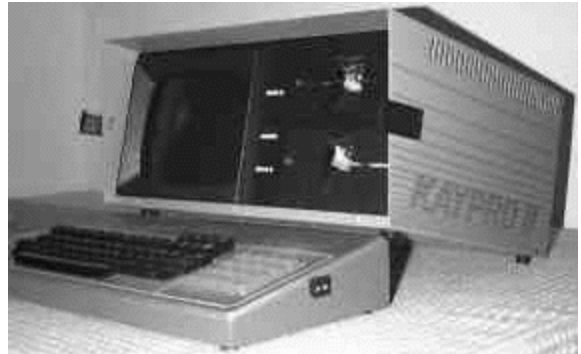
A Kaypro-2 "portable" computer this had a whopping 64k of RAM, two floppy drives and a gigantic 9" green screen. This "portable" weighed in at a mere 26 lbs!
