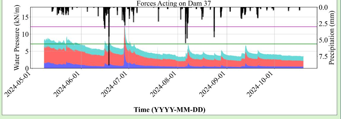
Fig. 4: Time series of the principle forces acting on the four studied beaver dams, from May to October 2024, in relation to precipitation events (black bars). The solid horizontal lines indicate the upper (pink; saturated) and lower (green; dry) beaver dam weights estimated from field measures, which is the primary resisting force. Wave pressure was not >0.03 kN/m and is so not shown.
