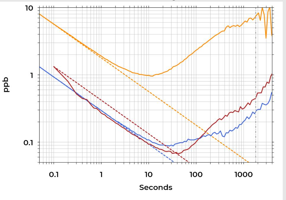
Figure 3: Allan deviations (Allen, 1966) computed to a 4-hour interval for all analyzers. The TGA instruments exhibit deviation smaller than the 10 Hz noise floor out to 30 minutes indicating stability for EC flux calculations.
