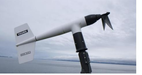
Damaged and misaligned RMY5106<sup>1</sup>
