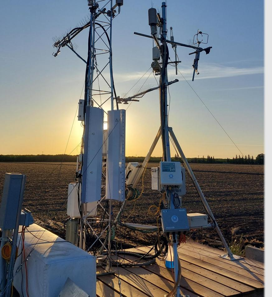
Figure 5: Test site equipment. TGA310, TGA320, TGA200A, CSAT3B, IRGASON, LI-7700, LI-7500, Young 81000RE, CR6, radiometers, soil sensors, etc.
