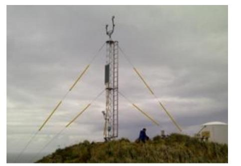
Both RMY5106 and 5108 are operational or the U-arm on the 10m tower<sup>1</sup>
