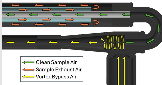
Figure 10: The external intake line houses a 4 m multi-layer dryer structure with a Nafion membrane tube at the center.
