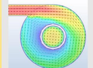
Figure 9: The vortex air cleaner reduces filter maintenance without impacting frequency response. Airborne particles are thrown to the outside of the vortex and carried away while the sample tube pulls cleaner air from the center of the vortex. (Burgon, et al. 2015)
