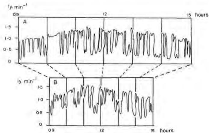
Fig. 2 Sample Recorder Traces; upper - Kipp; lower - Actinograph
