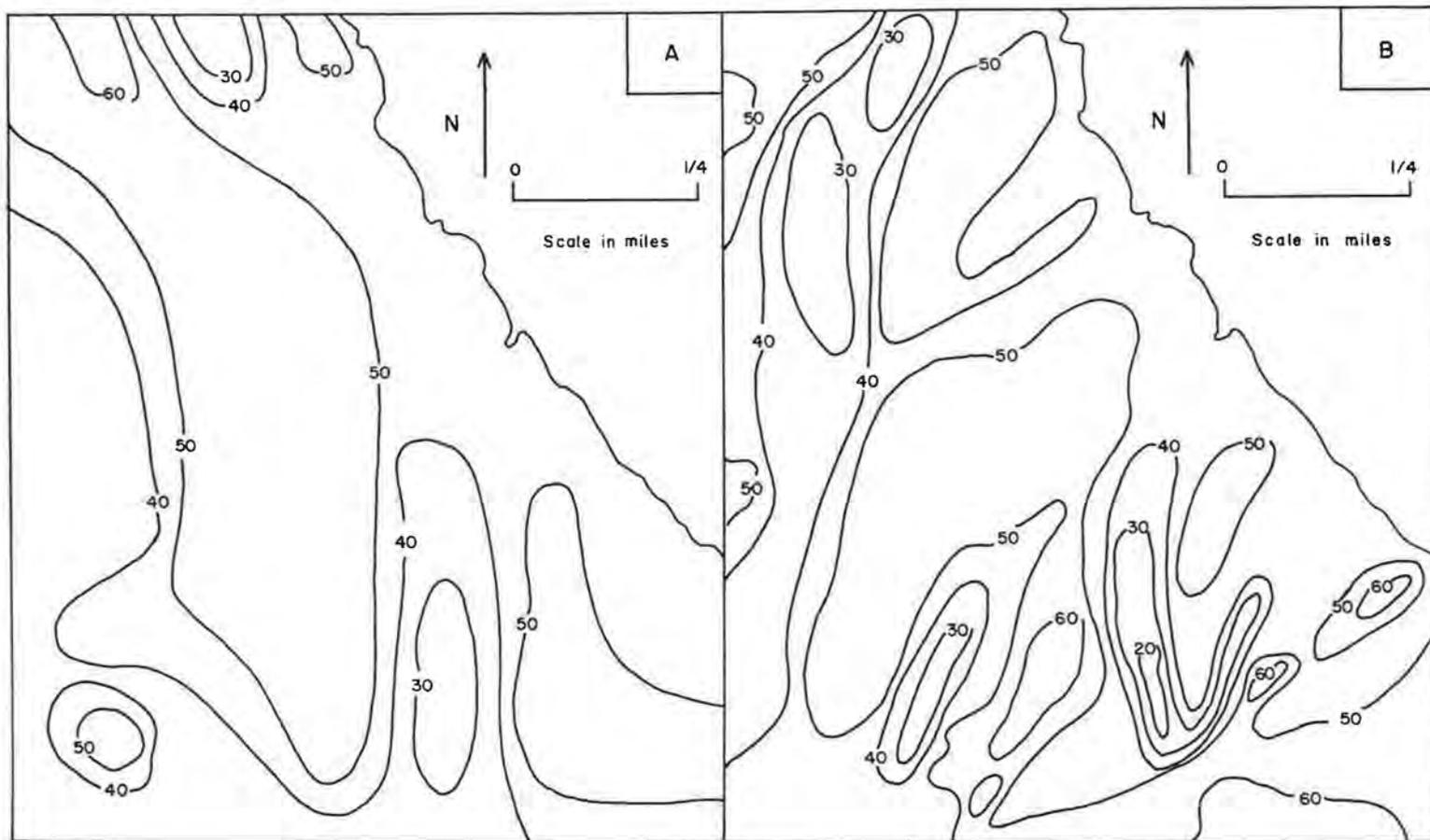
Fig. 3 Comparison of Grid Method (A) and Slope-facet Method (B) of Mapping
