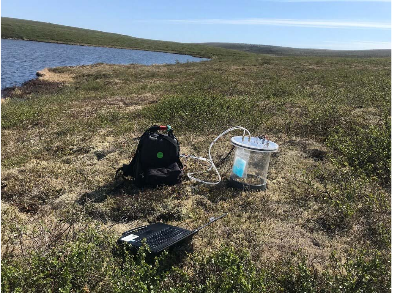
Image 4: Manual chambers. To measure CO 2 and CH 4 fluxes in harder to reach places, like this slope next to a lake, I use a manual chamber set-up. The manual chamber (right) is placed on an installed collar (image 3) and connected to a Picarro GasScouter (left) that analyzes the greenhouse gas concentrations within the chamber over time. I use a laptop to watch the fluxes in real-time and save a copy of the data. This is one of my favourite sites because of the beautiful lake view!
