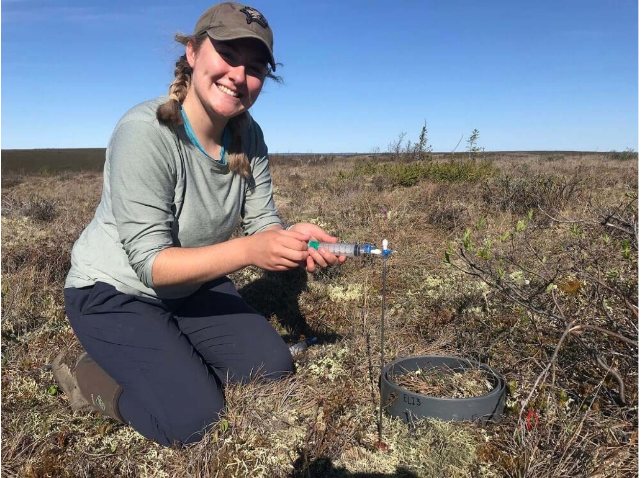
Image 3: Soil gas. I collect soil gas to understand below-ground processes that influence the fluxes I measure at the surface. At this tundra site, I am using a hollow stainless-steel tube connected to a plastic syringe to collect a sample of gas from below ground. I took this sample from beside a collar (right) that I have installed to measure above-ground fluxes. The collar ensures that I am measuring the same location since I return multiple times throughout the field season to take measurements. When I place the chamber on top, the collar allows me to create a sealed “mini-atmosphere” (see image 4) to measure gas fluxes. Photo was taken by Carolina Voigt.
