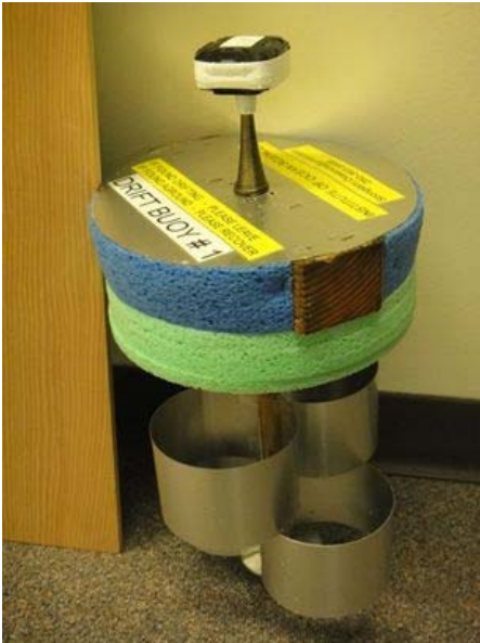
Low Cost Drifter developed at IOS
