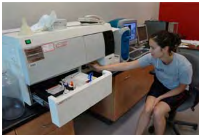
Figure 3: Fisheries and Oceans Canada technical expert Karen Scarcella operates a flow cytometer, which uses rapid electronic detection of light emission to analyze phytoplankton and bacteria in seawater samples from the Arctic Ocean. The speed, accuracy, and precision of flow cytometric analysis enable microbial cells to be surveyed and mapped at the high spatial resolution needed for detailed ecological study. Photo credit: William Li (Fisheries and Oceans Canada)
