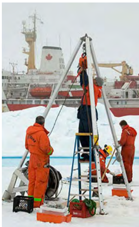
With the icebreaker CCGS Louis St-Laurent in the background, the science team sets up a through-ice mooring for year-round deployment of equipment that will measure such aspects of the ocean as its current, temperature and salinity.
