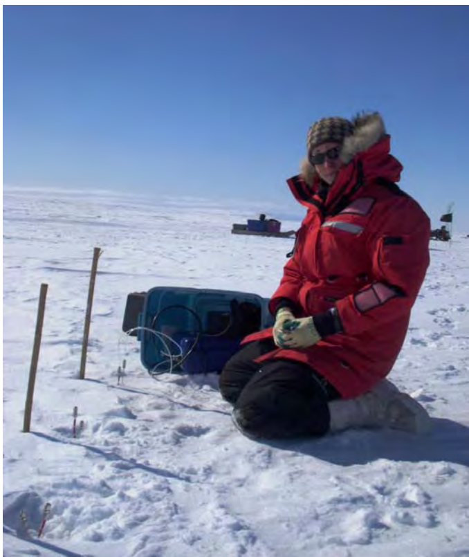
Kristina measuring the CO 2 concentration within "peepers", in situ semi-permeable gas samplers which have been frozen into the sea ice at the Allen Bay field site. (Photo: Cole Moszynski, June 2010).
