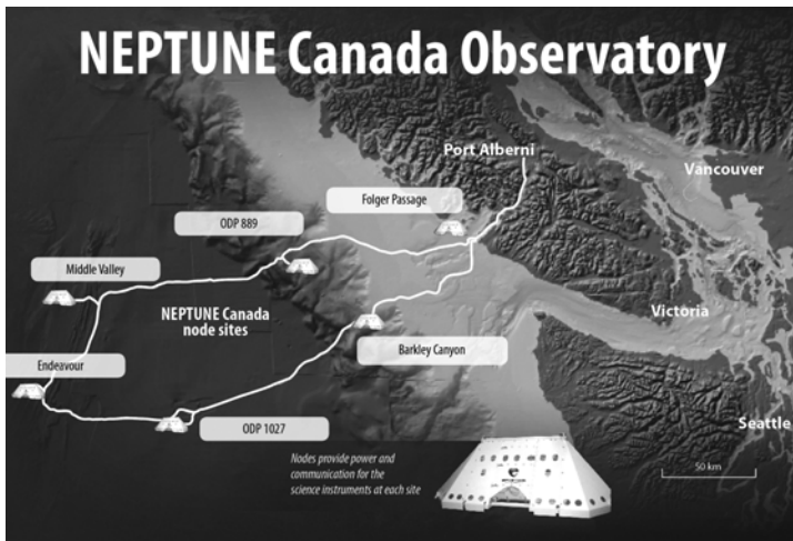
Figure 1: NEPTUNE Canada cabled ocean observatory showing 800km backbone cable route, node locations, Port Alberni shore station, and Victoria data centre. Also shown in colour on the cover page.
