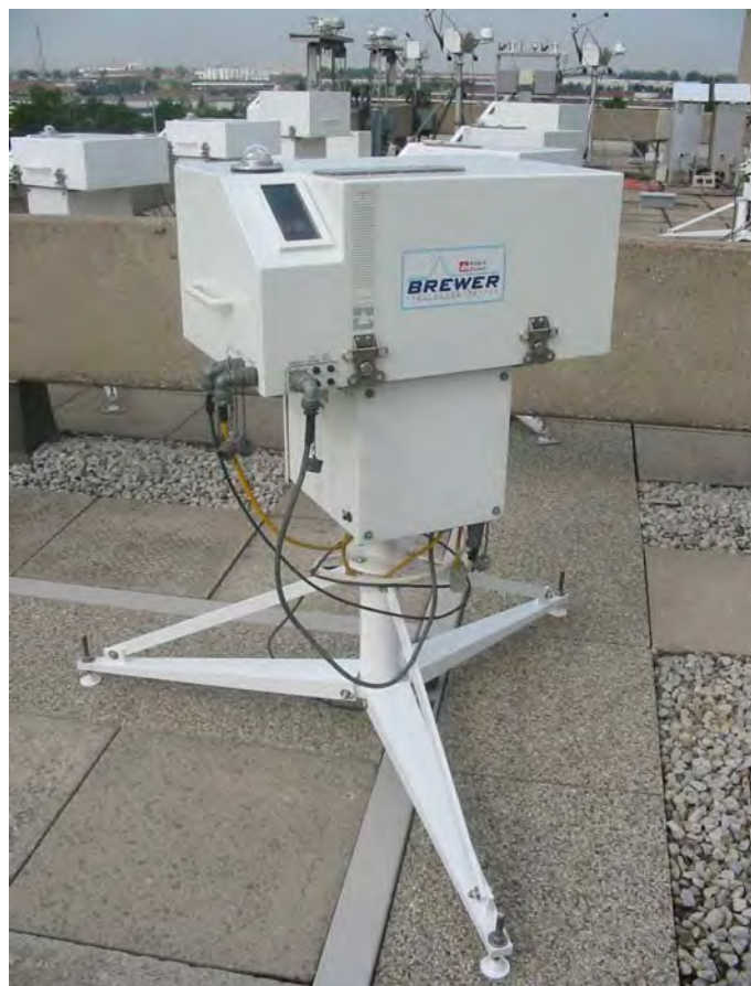
TEC. The corporate name was changed to Kipp & Zonen in Figure 3 : MKIII Brewer Spectrophotometer at Toronto (Devine 2004)
