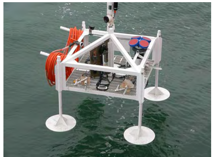
Figure 3: (Photo of VIP) A VENUS Instrument Platform (VIP), hosting a SBE CTD, an Aanderaa Optode, an RDI ADCP, and an ASL Zooplankton Acoustic Profiler. The wet-mate connector is attached to a 70m oil-filled orange hose and the Science Instrument Interface Module (SIIM, under the plate), which connects the VIP to a Node science port.
