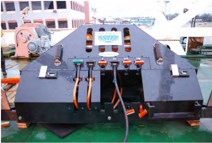
Figure 2: (Photo of black Node) The VENUS Saanich Inlet Node on deck before deployment in 2006. The upper Node pod (which can be recovered for servicing), contains the control systems and is connected to the back-bone cable with two wet-mate connects, one each for power and fibres, and hosts four side panel science ports with electrical wet-mate connectors.
