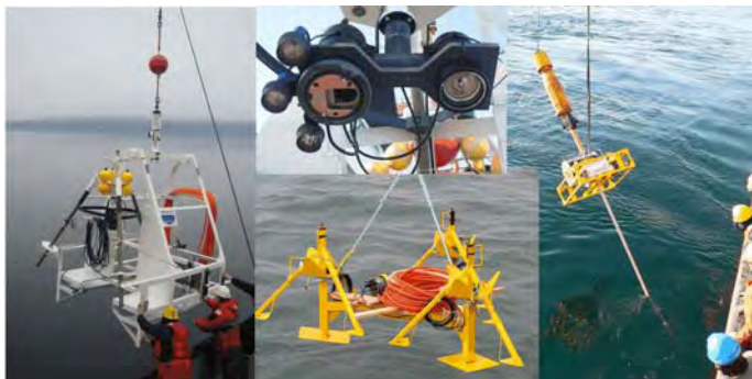
Figure 4: (Photo montage of camera, hydrophone, and SLIP) Specialized instrument systems include (left to right) the pan & tilt digital stills camera tripod and frame (camera and lights also shown in insert), one of the broadband hydrophone arrays, and a Seismic Liquefaction In situ Penetrometer (SLIP) which is seen here during deployment with a large weight that drives the instrumented tip 4 m deep into the Fraser River Delta sediments.
