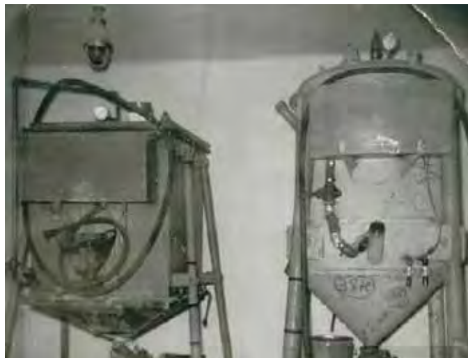
Figure 2. Gill Mark I and Mark II Low-Pressure Hydrogen Generators at Alert about 1963 (Courtesy of Monte Poindexter and the JAWS/HAWS web-site)
