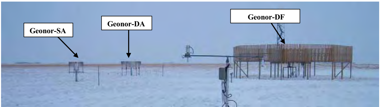
Figure 2: The Bratt's Lake intercomparison site containing Geonor T-200B precipitation gauges configured in a large octagonal double fence (right), a double Alter (center) and a single Alter (left) wind shield.
