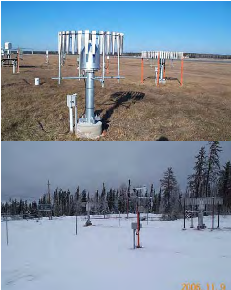
Figure 3: Top) Thunder Bay Geonor gauges with the single Alter shield in the foreground and the double Alter shield in the background. Bottom) Pickle Lake Geonors with the single Alter shield on the left and the double Alter shield on the right.
