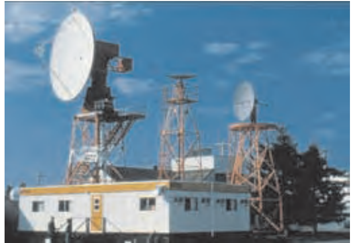
Figure 10: Radars used in AHP research and cloud-seeding operations, L-R: 10-cm S-Band polarization diversity radar, X-Band aircraft-tracking radar, 5-cm C-Band radar.
