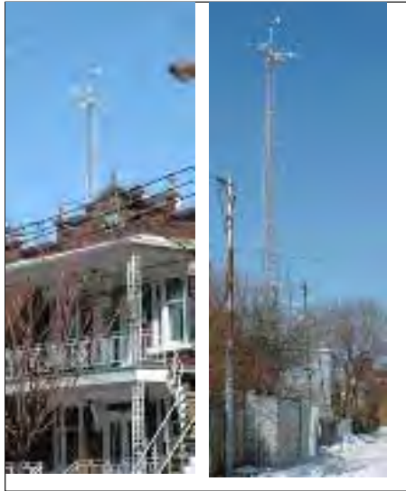
Figure 2. The 20-m telescopic meteorological tower with some of the instrumentation at the MUSE-2005 urban site in Montréal.
