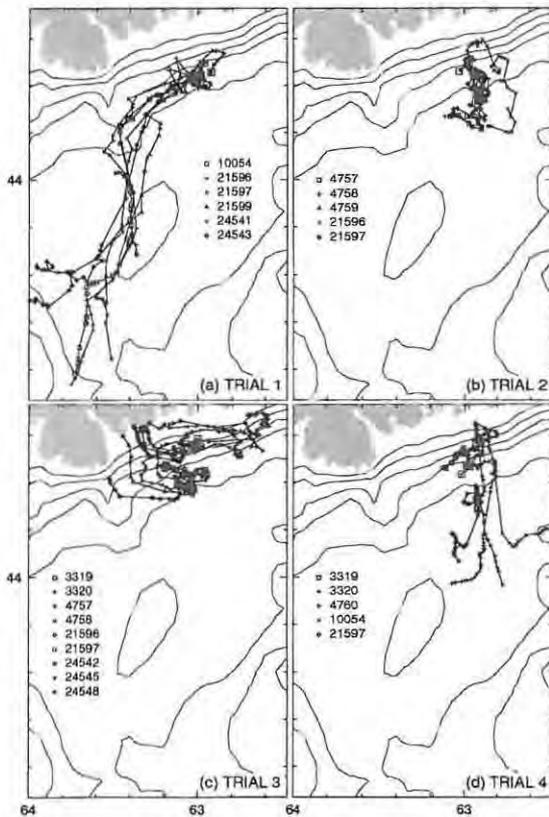
**Figure 5:** Positions of near surface drifters during the four field trials of the CANSARP Experiment, February, 1996. In (a) 24541 is a ballasted 6-person liferaft with a sea anchor and all others are SEIMAC ASTs; (b) all are SEIMAC ASTs; (c) 24542 is a ballasted 4-person liferaft (no anchor), 24548 is a dory with tethered AST, 3319 and 3320 are SEIMAC CASTs drogued at 15m; and all others are SEIMAC ASTs; and (d) 3319 and 3320 are drogued CASTs and the rest are ASTs.
