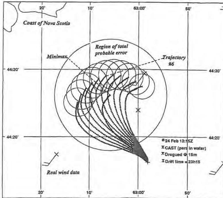
Figure 1: Sample CANSARP drift predictions for a CAST buoy. The 11 trajectories and their end point errors are calculated based on interpolated winds, currents, and estimated uncertainties in the leeway factors and angles; trajectory #6 is considered most likely. The larger circle represents the region of total probable error, which encompasses all of the trajectory end points and their errors (Verner, *et al.*, 1998).
