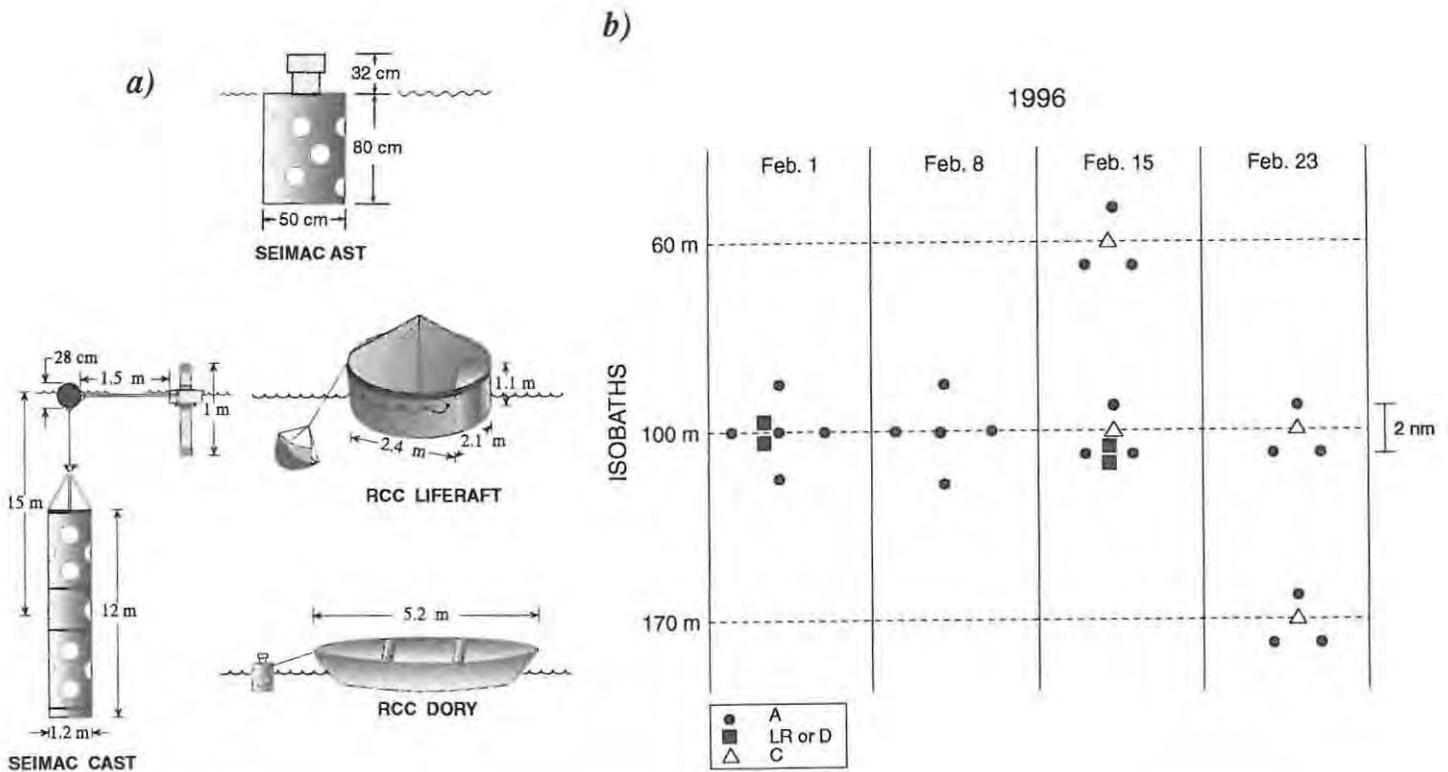
**Figure 3:** a) Schematic diagram of four classes of drifters used in the CANSARP field experiment. b) Drifter deployment patterns for four weekly trials on the Scotian Shelf during February, 1996. "A" stands for a SEIMAC AST; "C" for a SEIMAC CAST; "LR" for a 4- or 6-person life raft, and "D" for a 5.2m dory.
