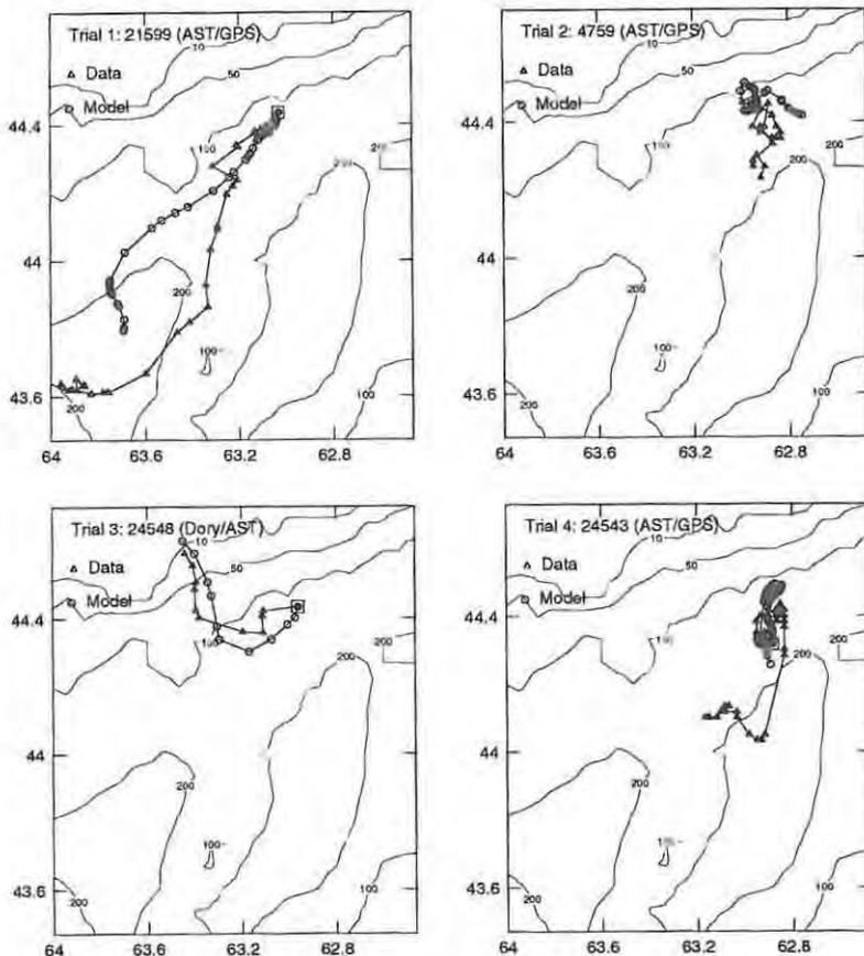
**Figure 7:** Typical observed and predicted drift trajectories during the CANSARP field experiment. The observations (predictions) are indicated by triangles(circles). The low-resolution (35-km) CMC winds were used and the baroclinic background current is included in the model.
