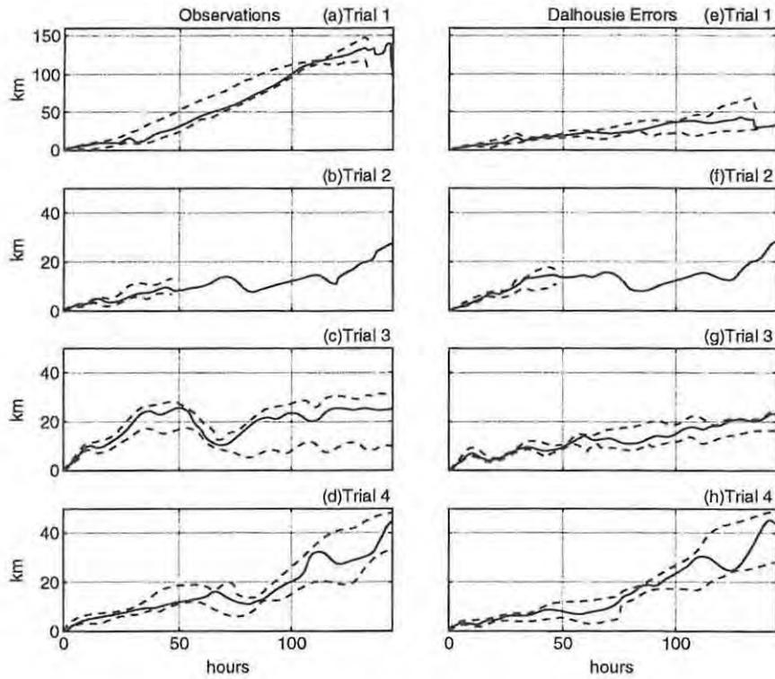
**Figure 8:** Drifter displacements with respect to their initial positions (a-d: left panels) and predicted positions (e-h: right panels). The solid line shows the time-varying radius of a circle which encompasses 50% of the drifters; the lower and upper dashed lines represent the 25% and 75% quartiles, respectively.
